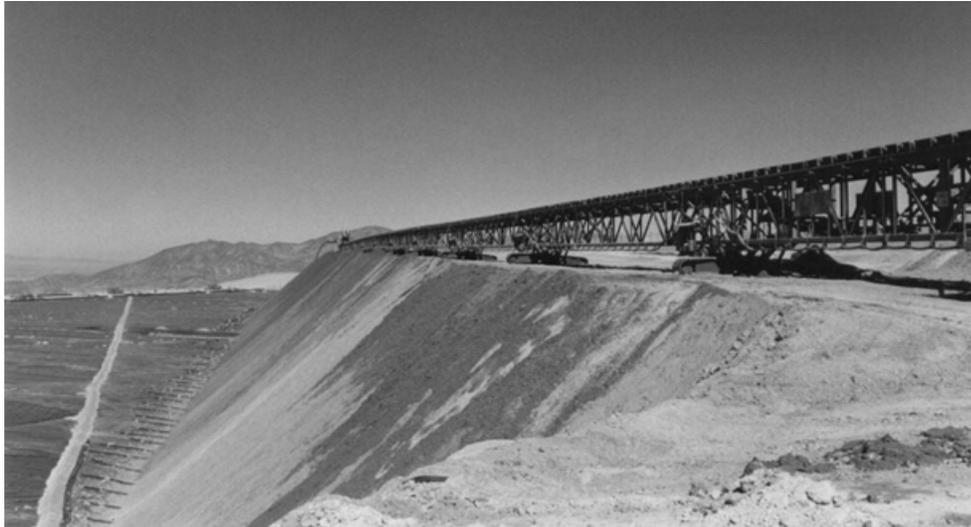
**Figure 8** Rahco stacker building a 12 meter lift by tripping the ore over the advancing edge. The stacker can climb ramps and turn sharply to fit project requirements.
