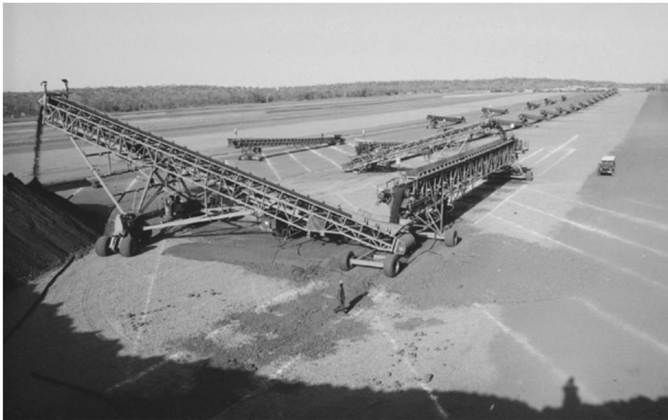
**Figure 7** Stacking system for capacity of 10,000 tonnes ore per day. Elements include stacker with extendable stinger; follower conveyor; cross conveyor; and several grasshopper conveyors.
