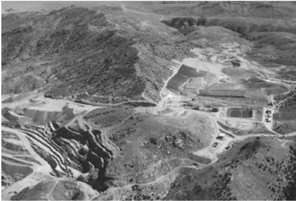
**Figure 2 Heap leach installation at Mineral Ridge, Nevada.** The open pit mine is shown on the left. On the right is a two million ton heap of crushed, conveyor-stacked ore placed on a plastic-lined leach pad. Pregnant and barren solution storage ponds are located downslope from the heap. Buildings include process plant, laboratory, maintenance shop and administration offices. Photo courtesy of Tom Nimsic, American Au/Ag Associates.
