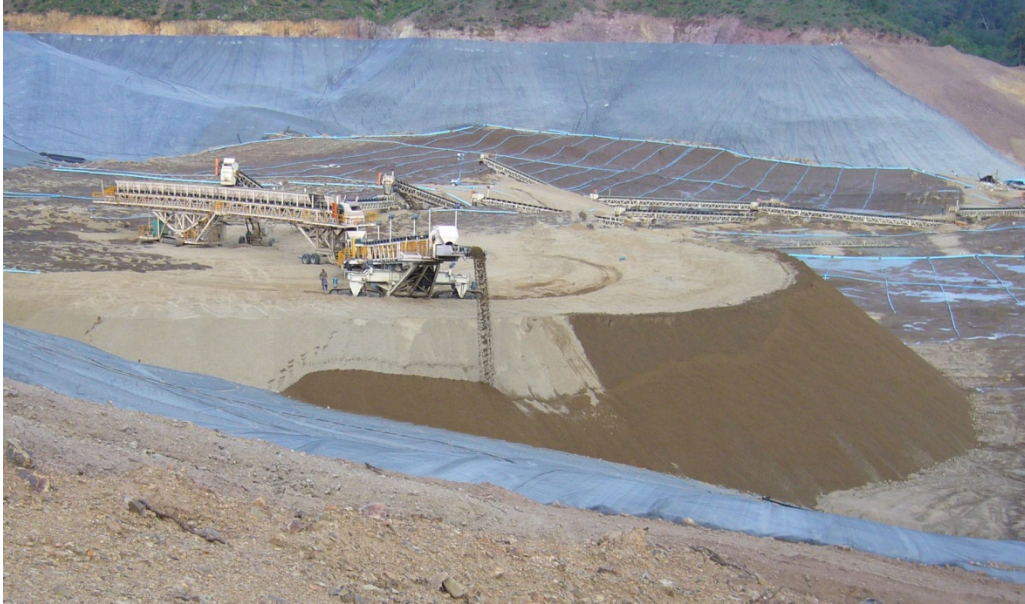
Figure 4: Top advance stacking of a 12,000 tonne/day heap
