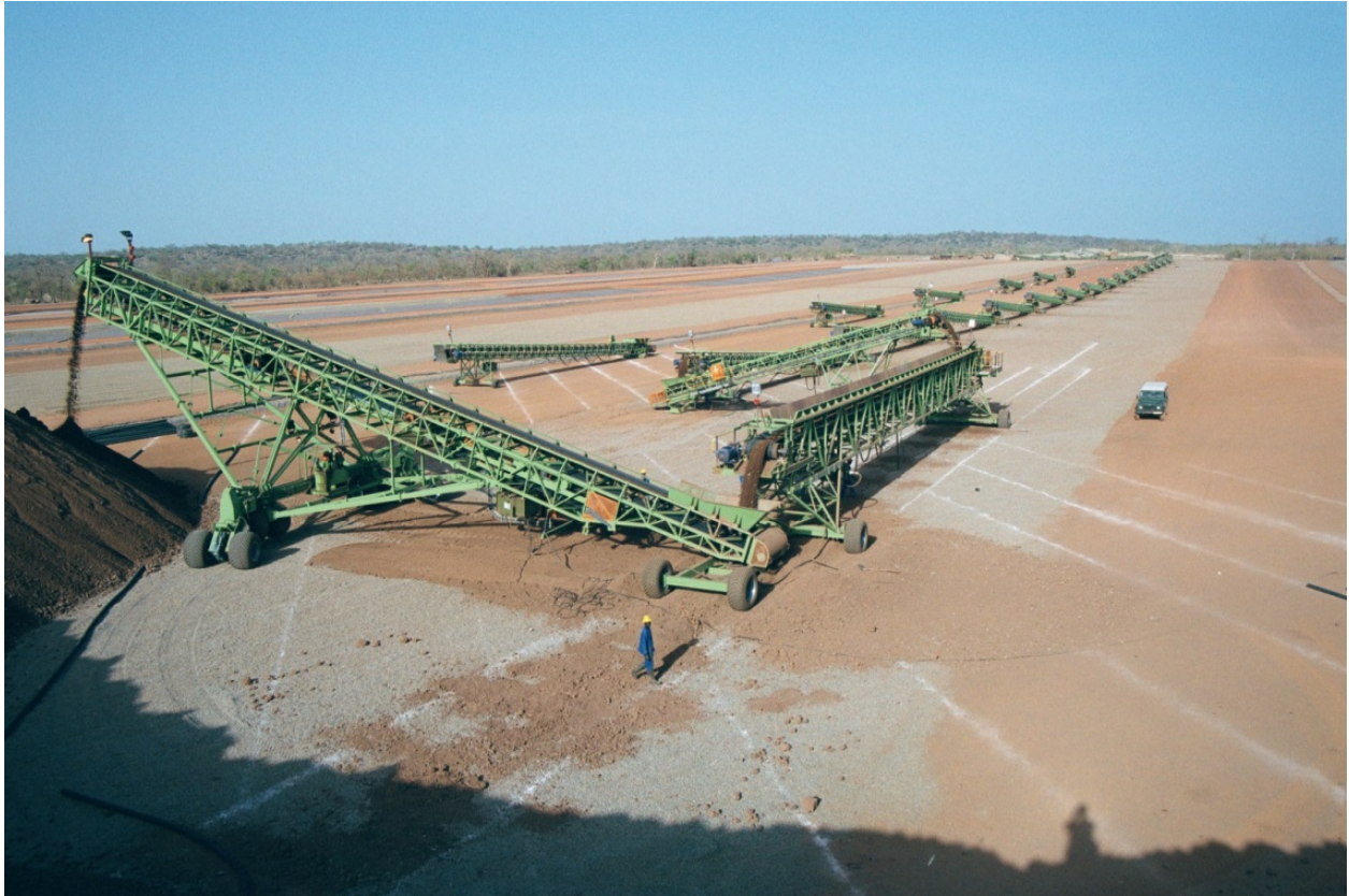
Figure 3: Retreat conveyor stacking system at Yatela, Mali
