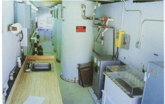
MODEL 20 CARBON ADSORPTION-DESORPTION-RECOVERY PLANT. 90 US GPM (20 CU M/HR) FOR PROCESSING 300-600 TONNES OF GOLD/SILVER ORE PER DAY.
