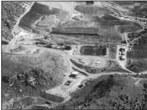
Figure 11.3-1 Heap leach installation at Mineral Ridge, Nevada
